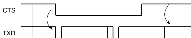
Figure 31-21. Transmitter Behavior when Operating with Hardware Handshaking
